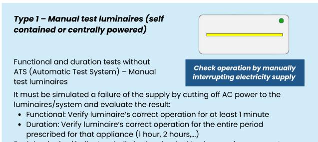
Each luminaires' indicator shall also be checked to show main power restore and battery charging
